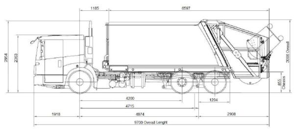
9.7m Heavy Rigid Rear Load Waste Collection Vehicle specifications
